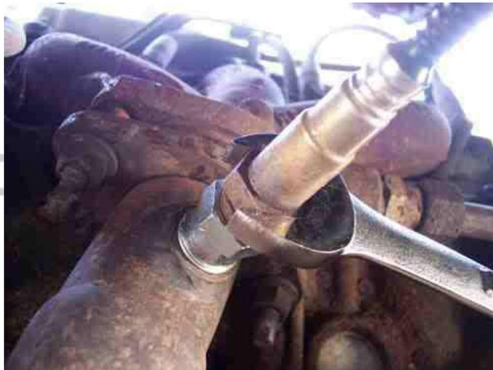
5. Reconnect the negative battery cable. Re-enter any codes. It may take a few days of driving for the ECU to relearn the new sensor position. It is okay if the check engine light comes on while the ECU relearns.
