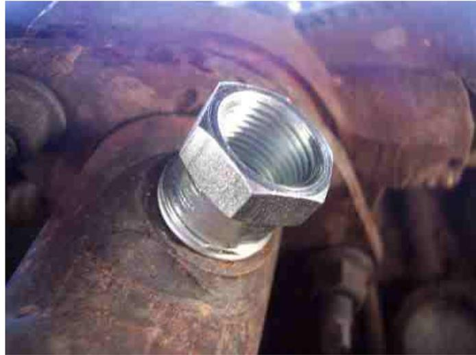
4. Thread the extender into the exhaust, in place of the sensor. Tighten to 50 Nm (37 ft-lbs) maximum. If a torque wrench is not available, tighten until the compression washer starts to crush.
