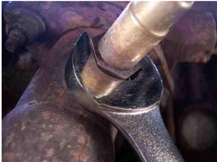
3. Thread the extender into the exhaust, in place of the sensor. Tighten to 50 Nm (37 ft-lbs) maximum. If a torque wrench is not available, tighten until the compression washer starts to crush.
